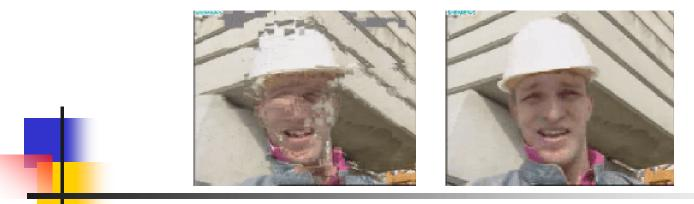
Error robustness for Internet packet loss using Unequal Packet Protection with a non-scalable MPEG coder (left) and an FGS MPEG-4 coder at 330 kbit/s (right) where the enhancement layer is completely lost.
