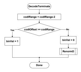
Figure 9-6 – Flowchart of decoding a decision before termination
