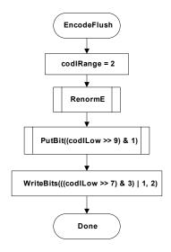
Figure 9-12 - Flowchart of flushing at termination
