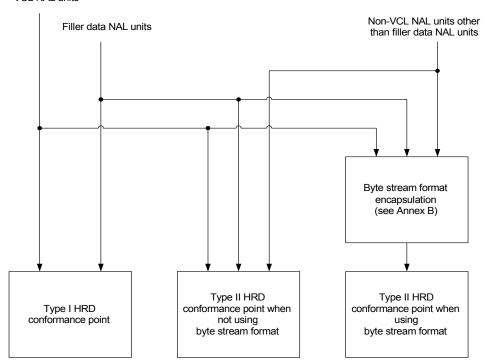
Figure C-1 - Structure of byte streams and NAL unit streams and HRD conformance points
