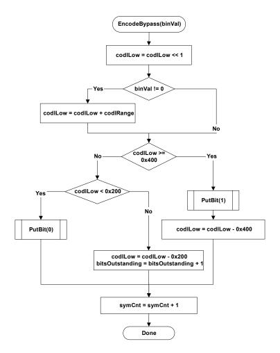
Figure 9-10 - Flowchart of encoding bypass
