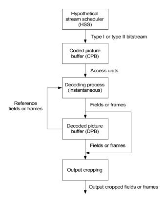
Figure C-2 – HRD buffer model
