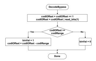
Figure 9-5 – Flowchart of bypass decoding process
