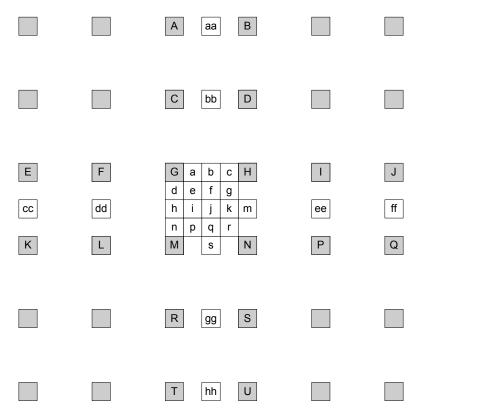
Figure 8-4 – Integer samples (shaded blocks with upper-case letters) and fractional sample positions (un-shaded blocks with lower-case letters) for quarter sample luma interpolation.
