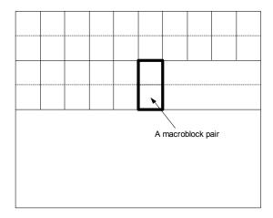
Figure 6-4 – Partitioning of the decoded frame into macroblock pairs.
